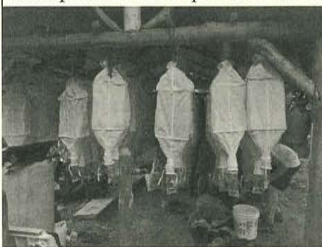
Mini-Winkler funnels hanging from roof beams
